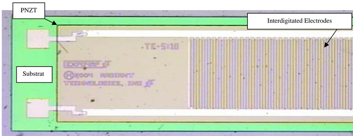
**Photomicrograph of the Bond Pad End of the Cantilever**
