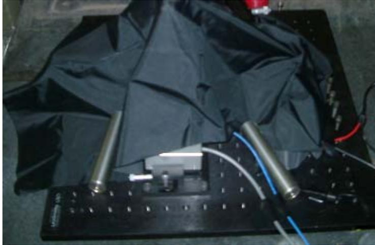
**Shrouded Optical Test Path**
