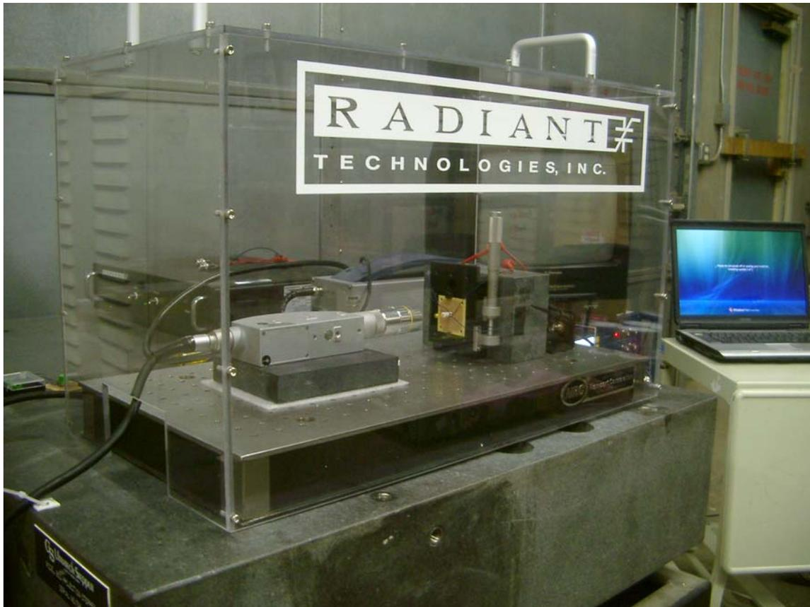
**Precision Displacement Test Stand with Polytec Laser Vibrometer
