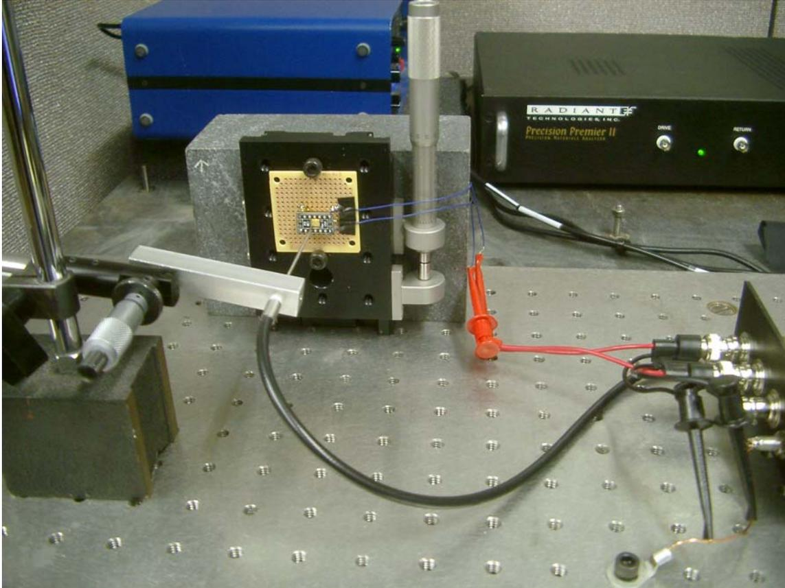
**The Brick with a Sample and an MTI Photonic Sensor on the PDTS
