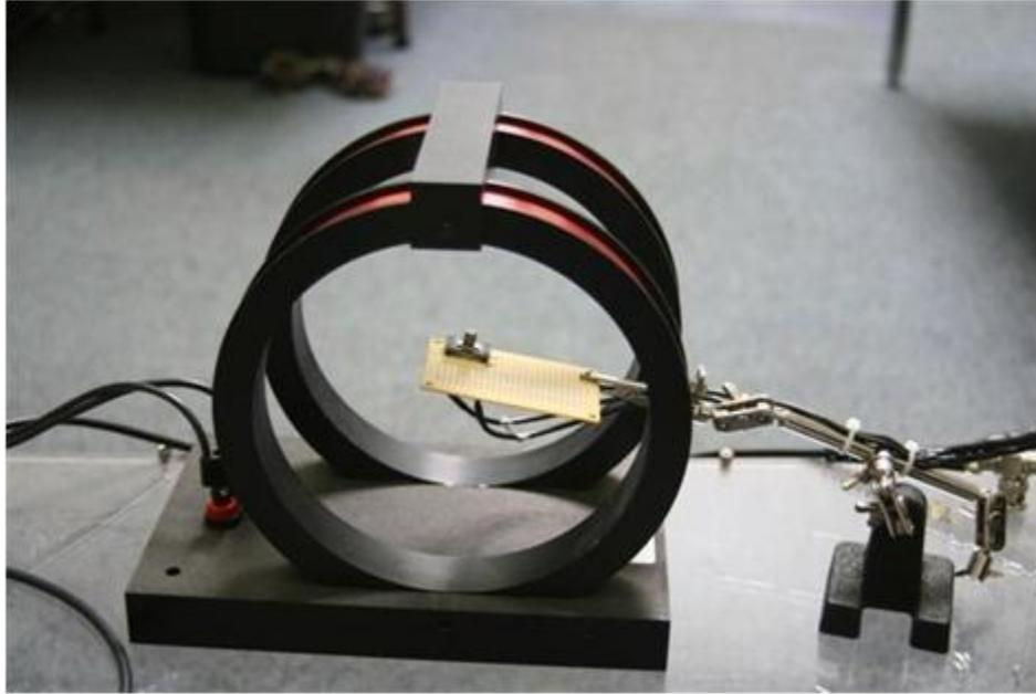
**Fig. 10b:** Reference Sample in Helmholtz Coil.
