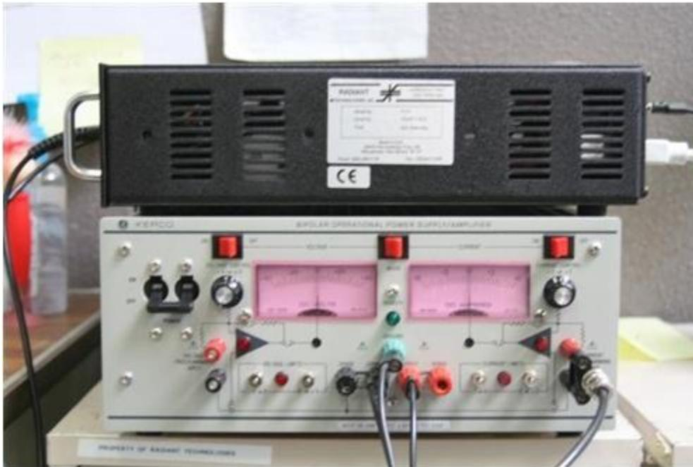
**Fig. 10a:** Precision LC and Kepco 36-6 current amplifier.
