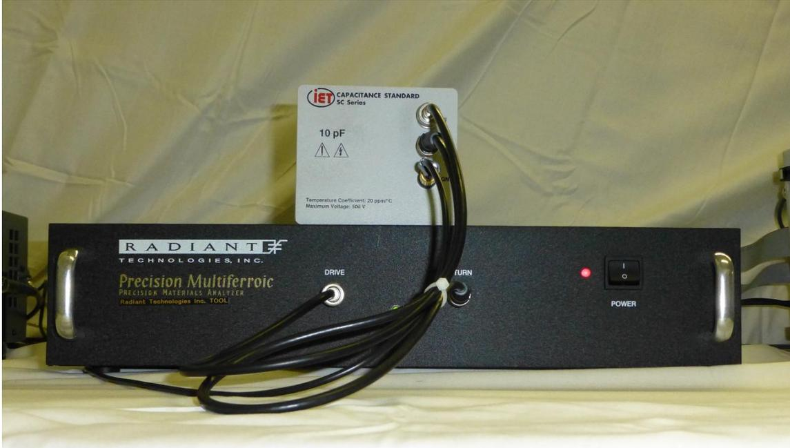
**Figure 4:** Test Fixture for the small charge measurements.
