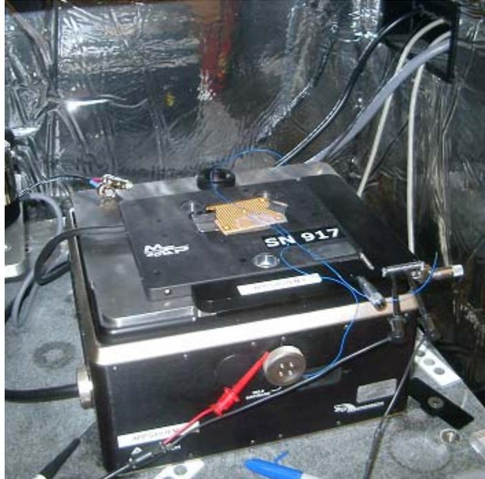
**Perf Board and Sample on the AFM Base
