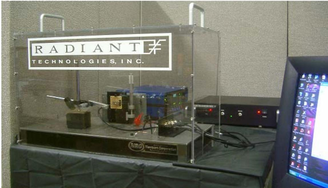
**Precision Displacement Test Stand
