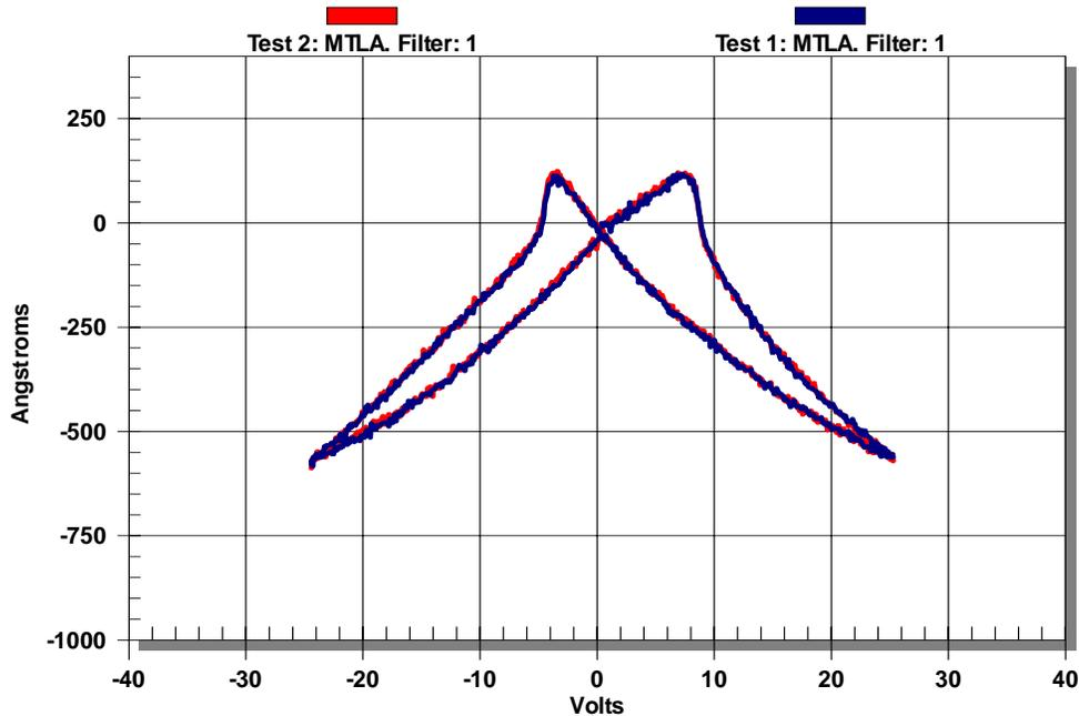
4mm Sensor Die Bending Moment Measured with SIOS Laser Vibrometer
