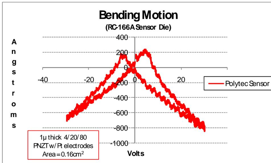
**4mm Sensor Die Bending Moment Measured with Polytec Laser Vibrometer**
