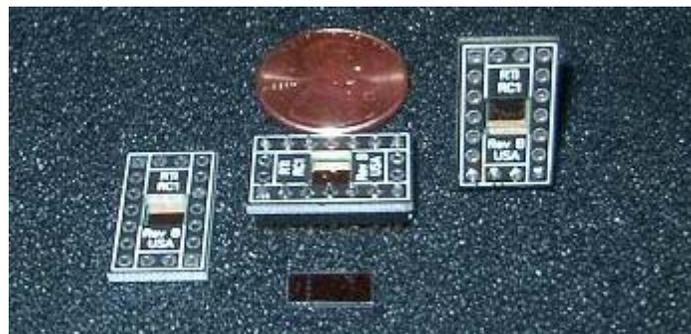
**4mm Sensor Die and PC Board Carrier**
