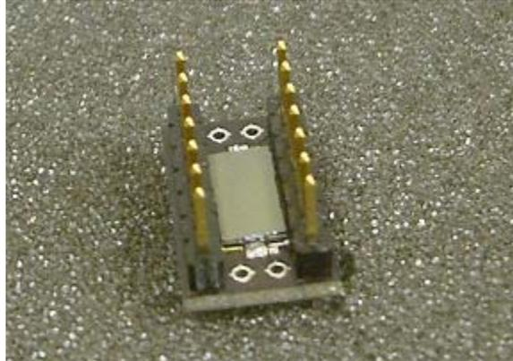
**4mm Sensor Die on its PC Board Carrier**
