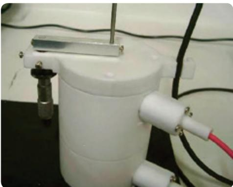
Figure 3 shows the HVDM and MTI2000 control unit. A 2032 sensor wand is mounted on the HVDM.
