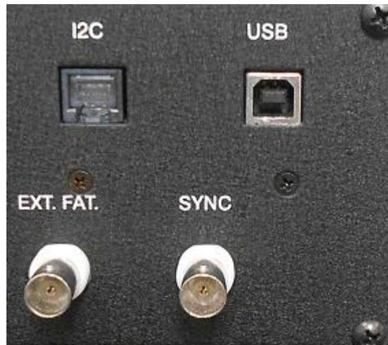
**Figure 11:** I<sup>2</sup>C port on the rear panel of a Precision Multiferroic Tester
