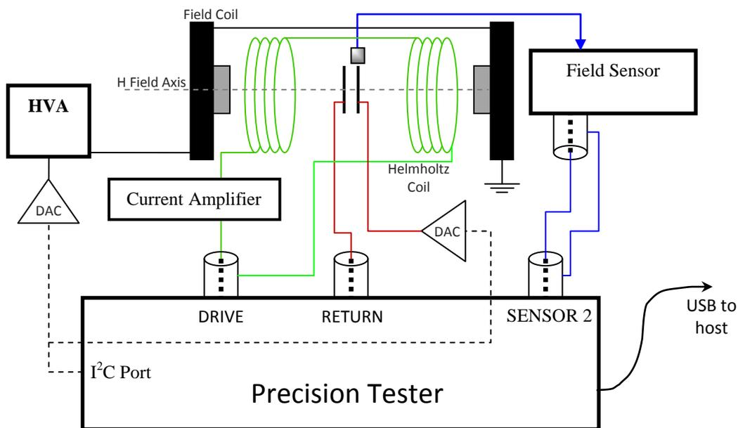
**Fig. 4:** The MR test configuration with DC field coil and sample voltage bias.
