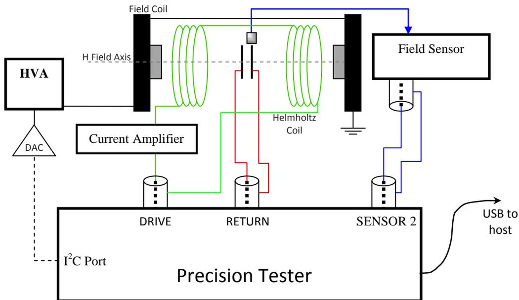
**Fig. 3:** Sensing magnetic field directly on Sensor 2.
