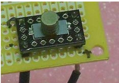
**Fig. 1:** Hand-built magnetolectric sensor
