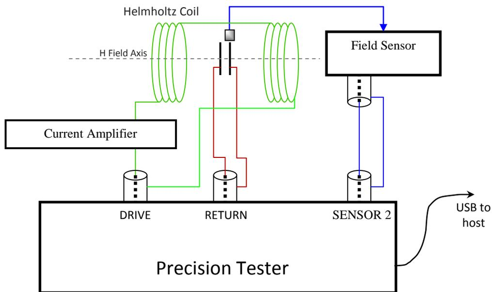
**Fig. 2:** The standard test configuration for the MR Task
