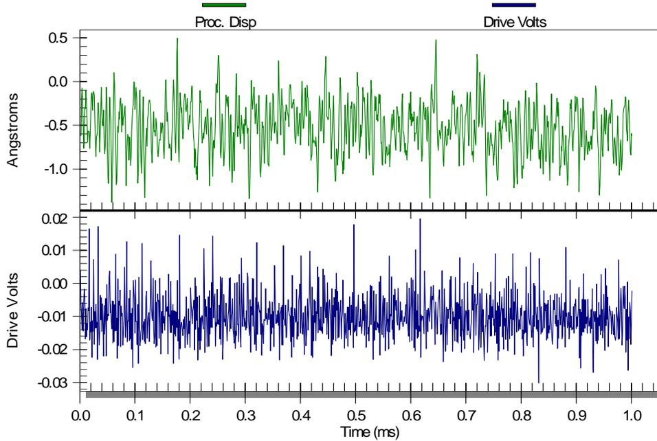
Drive Voltage and Displacement for Sensitivity Check
