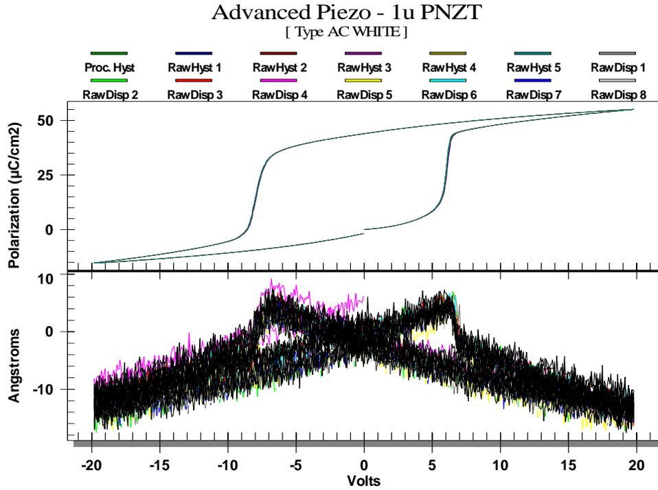
**Twenty Raw Polarization and Displacement Loops from Advanced PIEZO
