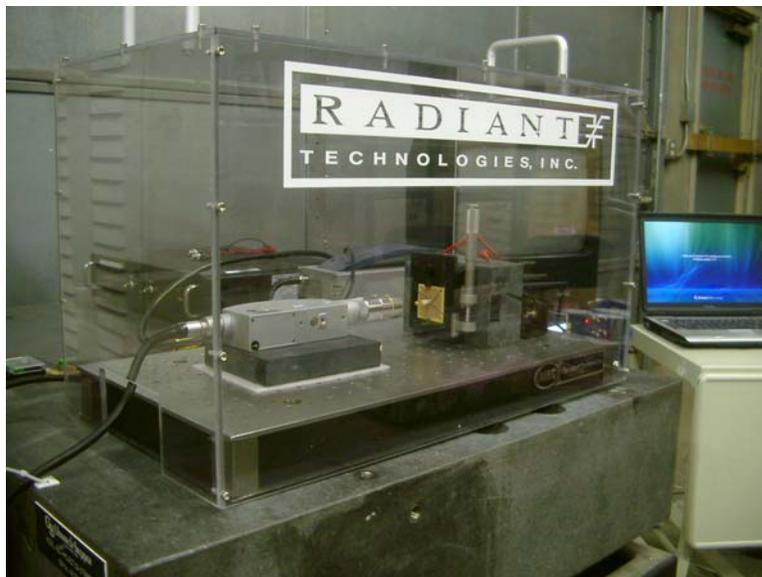
**The Laser Vibrometer and Sample Mounted on the PDTS
