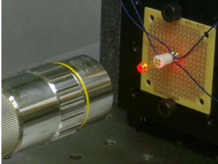
**TO-18 Header Mounted on the PDST Brick
