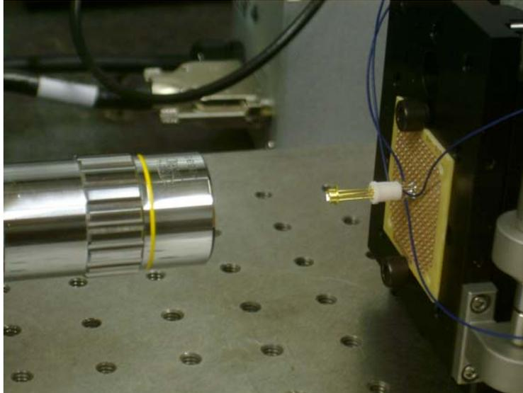
**TO-18 Header with the Capacitor Die in Front of Polytec Laser Sensor Head
