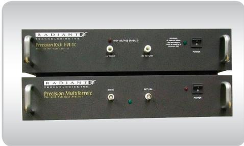
During normal operation, when a test is not being performed, the high voltage DRIVE and RETURN outputs of the Precision HVI-SC are disconnected from the HVA and connected directly to earth ground preventing any latent voltage from remaining on the sample.
