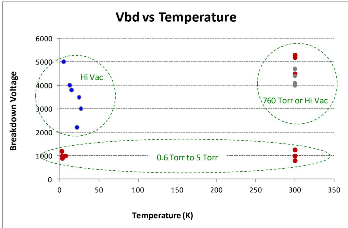
Fig. 3: All breakdowns in helium as a function of temperature.
