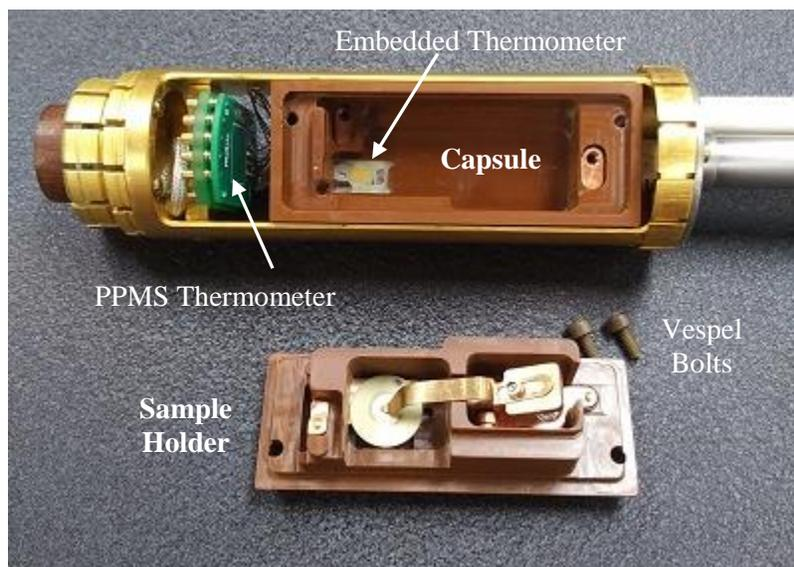
High voltage wires from the tester enter the Capsule where they connect with their internal terminals. The capacitor under test clips between a bottom Oxygen-Free High Conductivity (OFHC) copper square and a top spring loaded OFHC clip in the Sample Holder. The Sample Holder inserts into the fixture capsule and is secured with PEEK bolts. Pogo pins in the Sample Holder connect the sample to the high voltage terminals of the Capsule.
