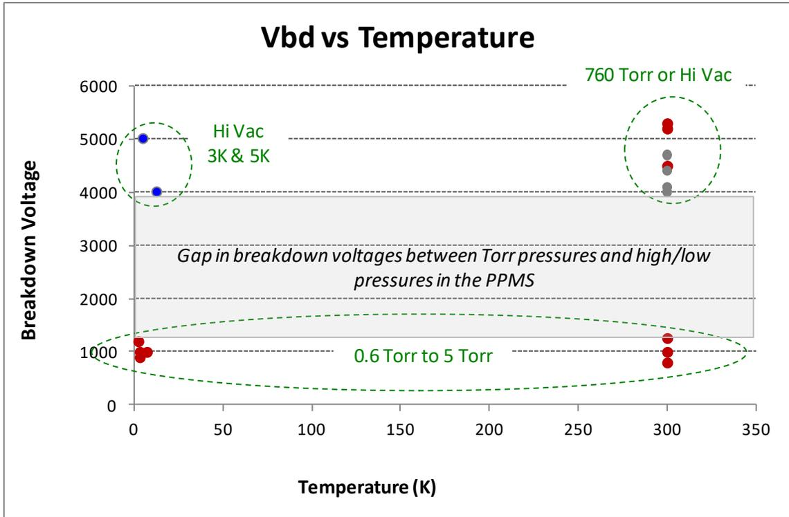
Fig. 4: All breakdowns in helium not associated with a rising sample temperature in high vacuum.
