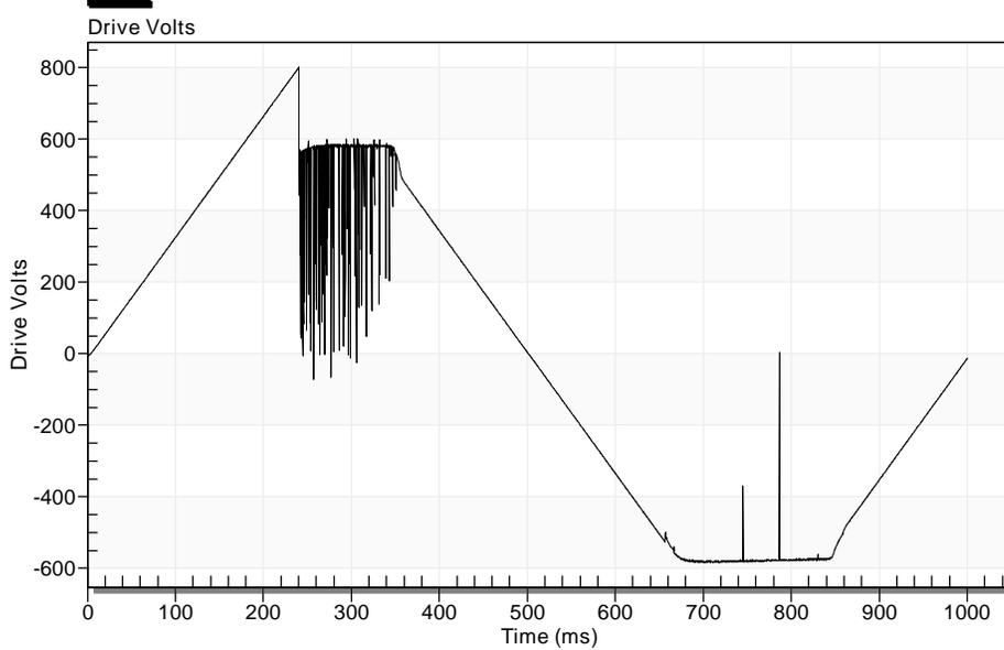
**Fig. 1:** Hard breakdown in 6 Torr 300 K helium
