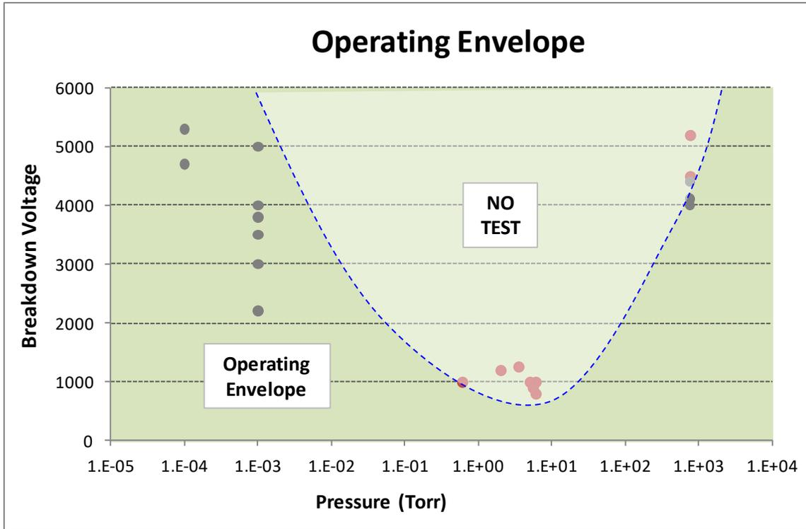
Fig. 6: Predicted Voltage-Pressure envelope for successful high voltage testing in the PPMS.
