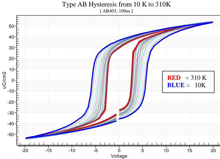
**Fig. 11:** 20/80 PZT Hysteresis vs Temperature.
