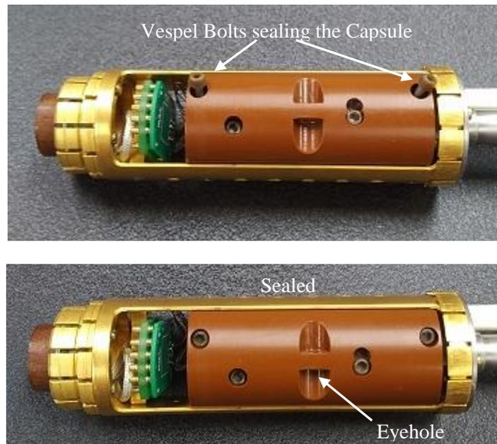
**WARNING:** Metal bolts *cannot be used* to secure the Sample Holder to the Capsule as they may reduce the voltage at which arcing occurs inside the fixture in low pressure helium. Please contact Radiant to replace missing PEEK bolts.
