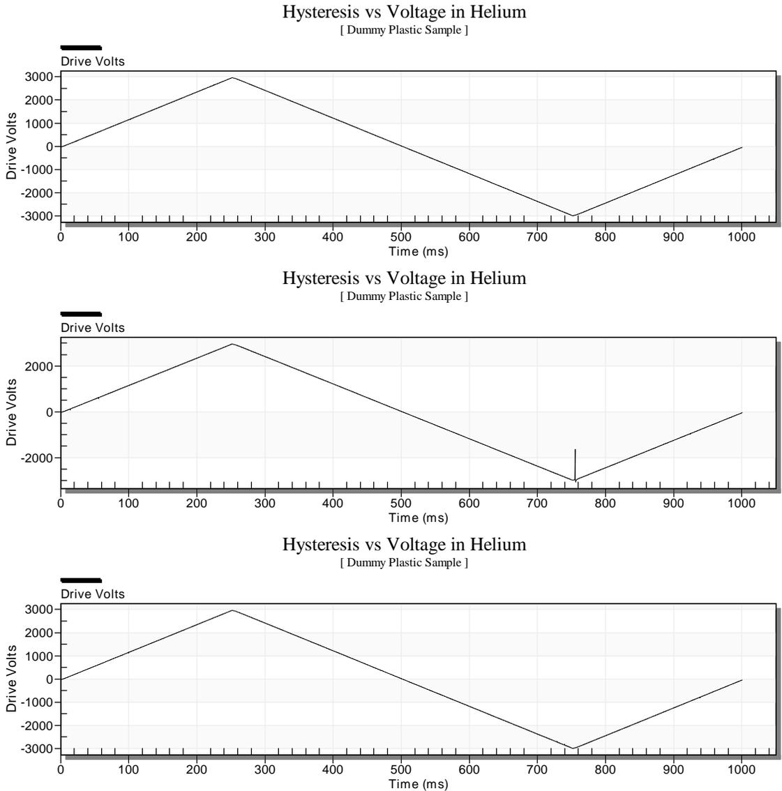
**Fig. 2:** One soft breakdown out of three tries in 1mTorr 26.4 K helium.
