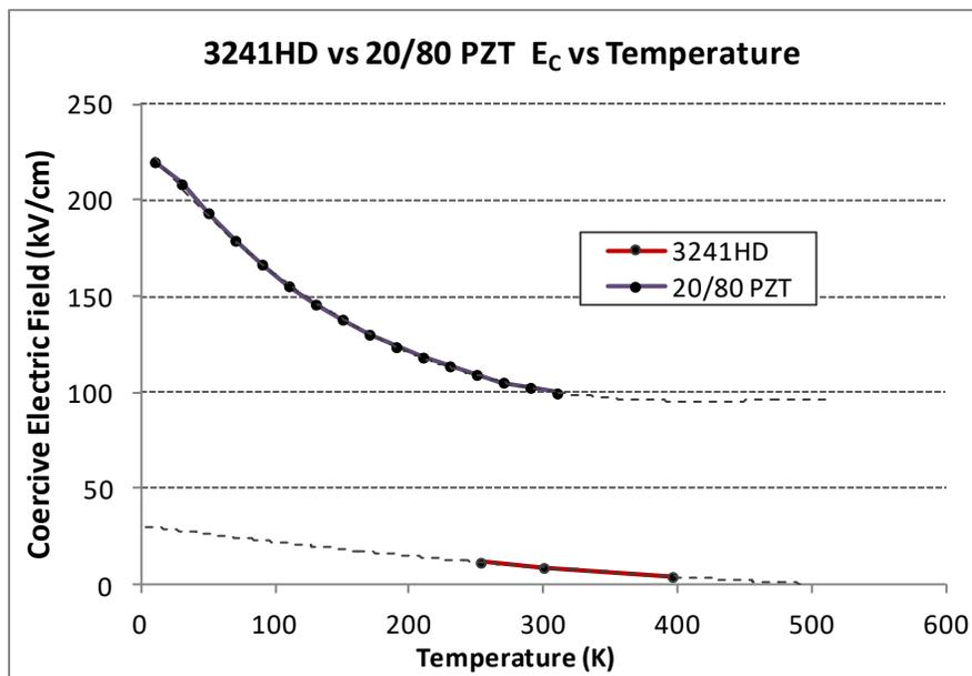
**Fig. 12:** Thin 20/80 PZT versus bulk 3241HD ceramic.
