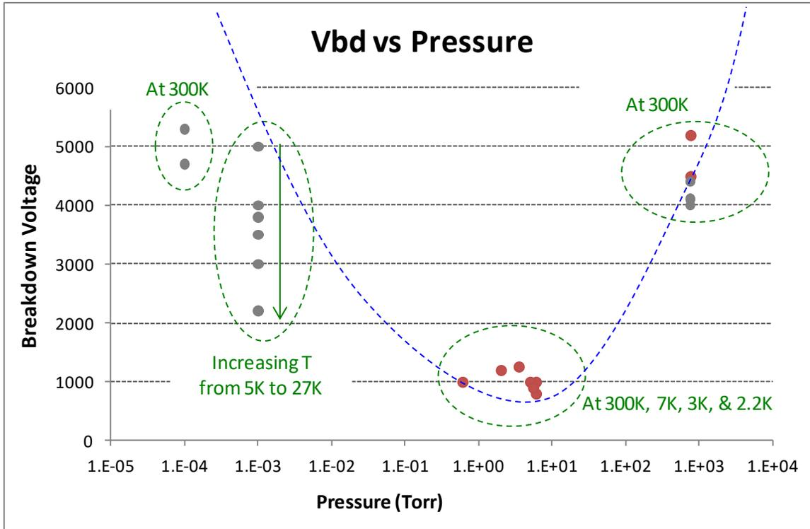
Fig. 5: All breakdowns in helium as a function of pressure.
