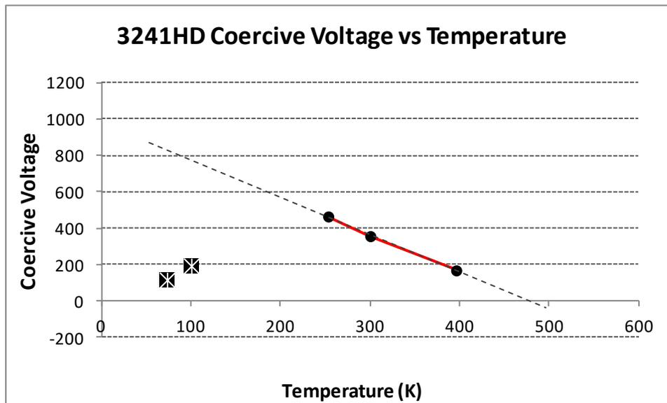
Fig. 10: Projected Hysteresis Coercive Voltage vs Temperature.
