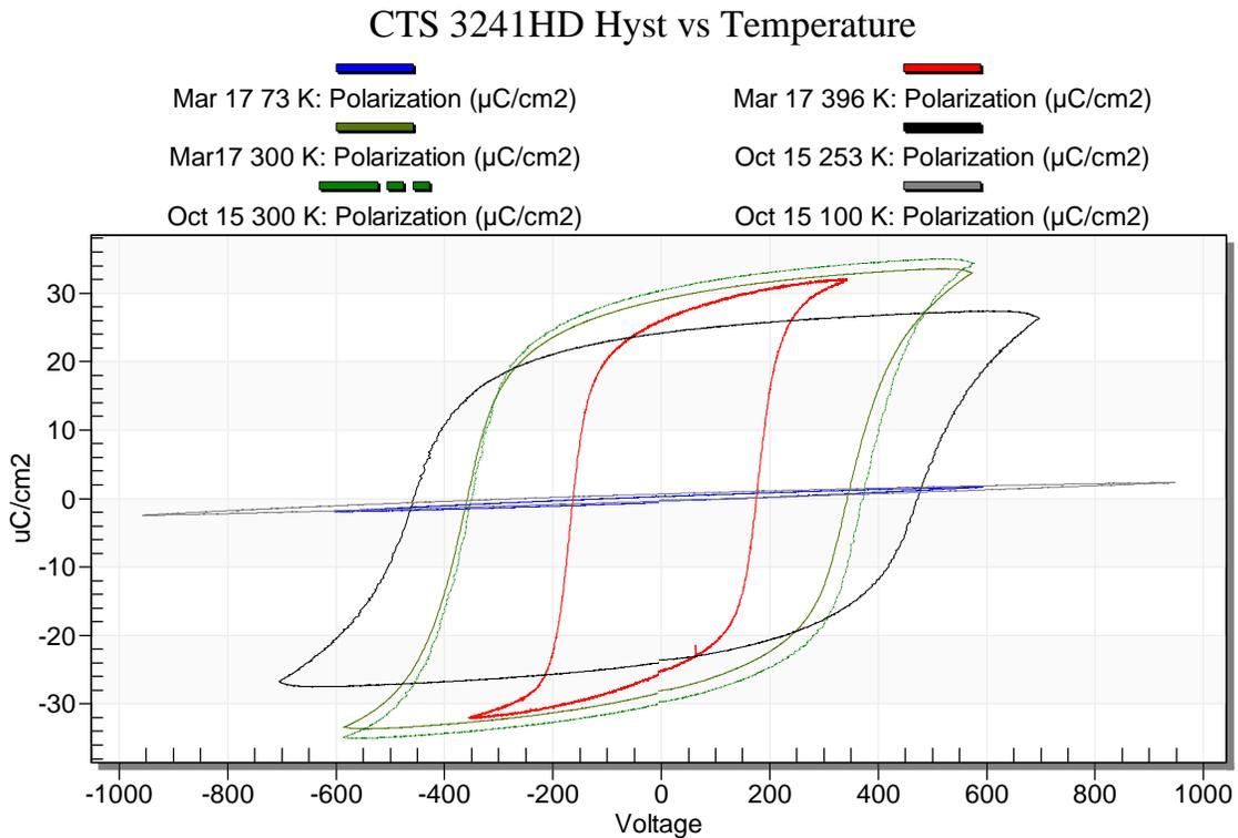
**Fig. 9:** Hysteresis measurement of 3241HD from 2015 and 2017.
