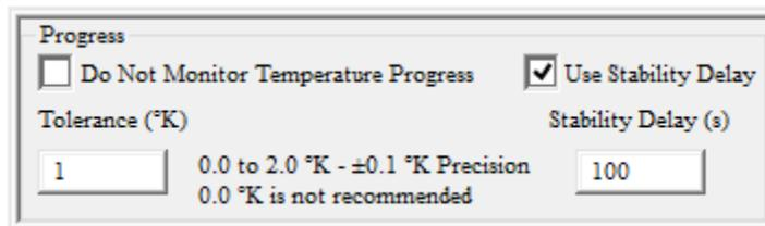
With the progress conditions set as in the image above, upon execution the Task will continue until the temperature has changed to the new value and has remained within 1 K of the assigned value for no less than 100 seconds. While waiting, the Task continuously reads and displays the temperature of the chamber. Since the Task does not exit until the newly assigned temperature has stabilized, the two parameters “**Current Set**
