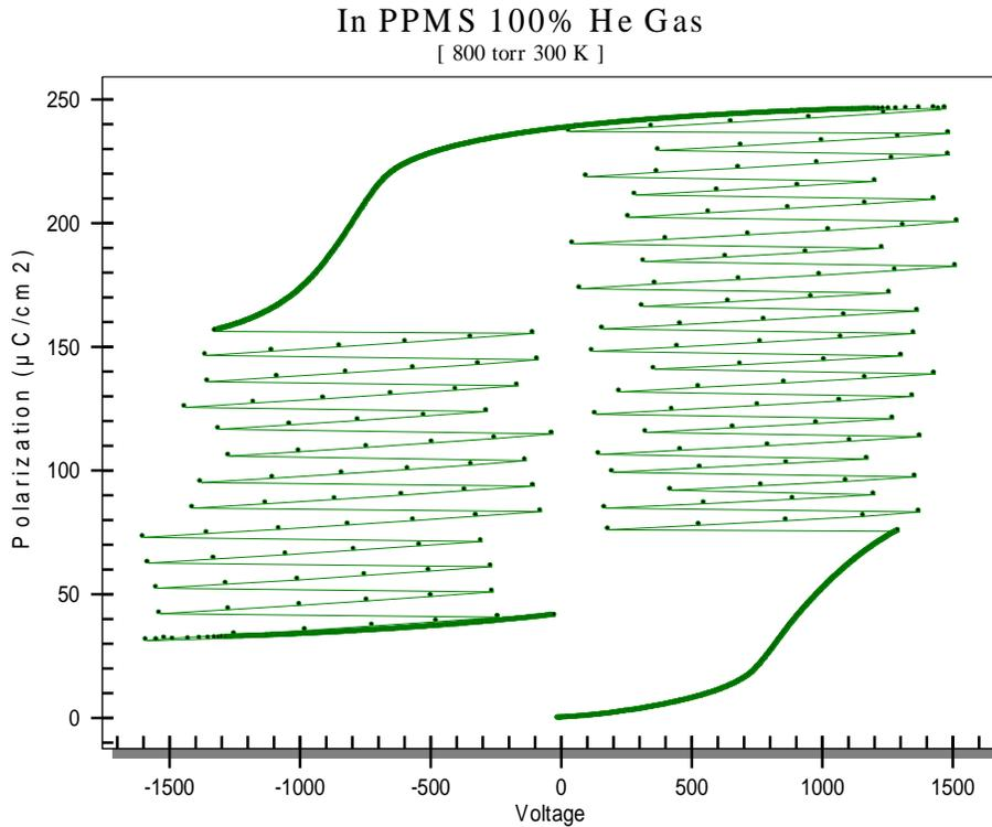
Note that the breakdowns in the plot above *where through the helium*. The sample remained undamaged despite the dramatic appearance of the plot. The voltage assigned for the test was simply above that which the helium could handle.
