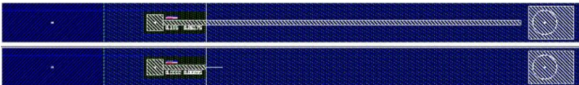
Fig. 9: Top-Standard Cantilever. Bottom-Same cantilever with 40,000 square micron actuator capacitor
