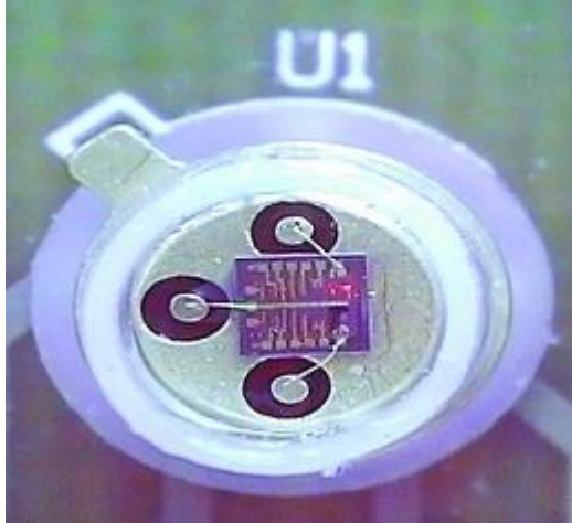
Fig. 6: Laser spot on 1µm-thick PNZT capacitor on test printed circuit board.
