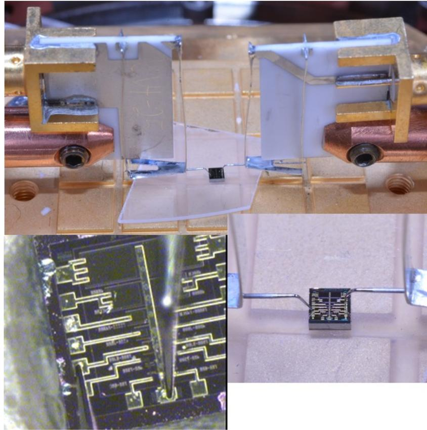
Cryogenic probe stations such as the Lake Shore Cryotronics Model CRX-4K permit testing of thin ferroelectric films on small substrates from 350 K or higher down to  $\sim 6$  K.
