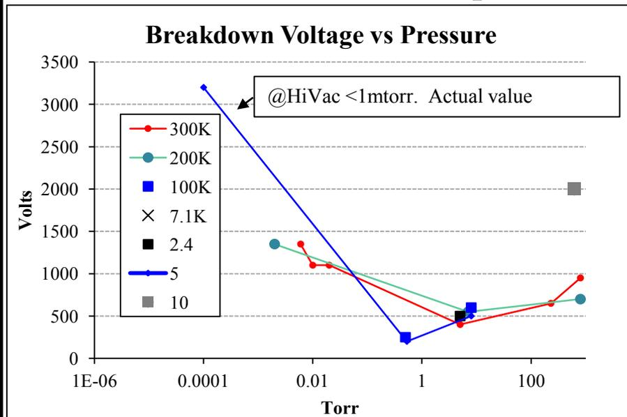
In the plot to the left, the lowest breakdown voltage for our tests occurs at roughly the same chamber pressure despite the different temperatures.
