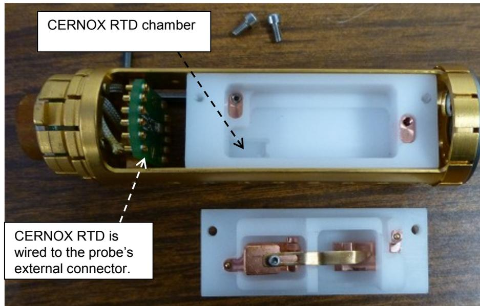
*Hanging in air, this fixture easily handles 10,000 volts. No so in the chamber in a helium atmosphere. There the breakdown can be as low as 400 volts!*
