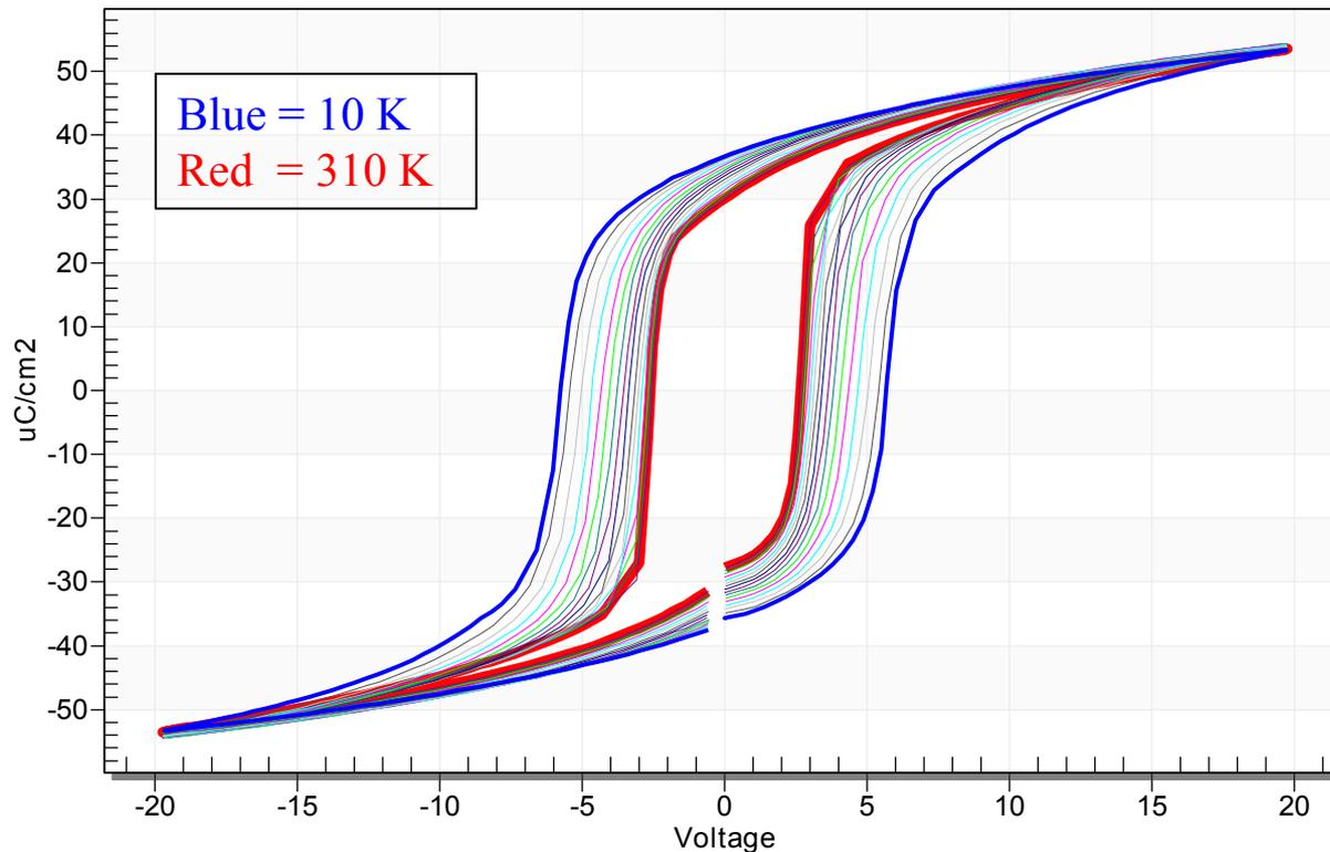
*The faster test period of 100  $\mu\text{s}$  prevented breakdown of the sample capacitor at 20 volts at room temperature.*
