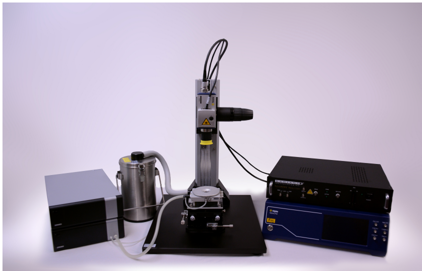
High-Resolution Angstrom-level Platform- PiezoMEMS Analyzer, VibroOne Laser and Temperature Stage -196 to 600C. Bundle measures piezoelectric coefficients and temperature
