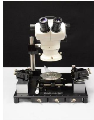
Probe station for the research of advanced active and passive components. Binocular and Trinocular stereo zoom microscope with 20X magnification (included wide field eyepieces), LED ring illuminator, precision x-y stage with isolated and shielded chuck, vacuum hold down and Z-lift.
