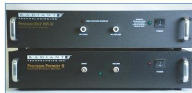
The Precision Premier II is an advanced tester that has a large test envelope in terms of frequency response, voltage range and accuracy.
