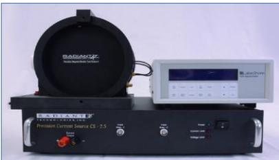
Radiant's Magneto-electric Test Bundle allows users to set DC Magnetic Fields across a sample using any coil and adjust those fields while a test progresses under Vision Software.
